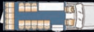
15 Passenger Aisle Facing with 72" Interior Luggage Rack 158" WB DRW
